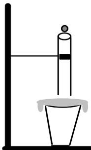
9. cup. Use these distances: 11 cm for a drop of 40 cm, 16 cm for a drop of 45 cm, 21 cm for a drop of 50 cm, 31 cm for a drop of 60 cm, and 41 cm for a drop of 70 cm (if needed) until the putty film breaks.
