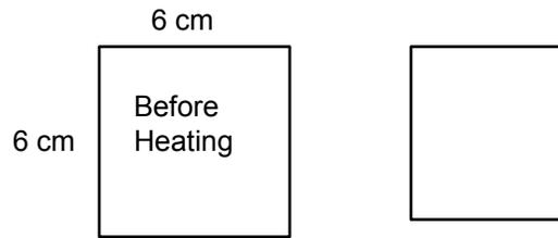
6. Using your skills in mathematics, calculate the rectangle that must be drawn on the second piece of PET plastic so that when it is exposed to boiling water, the resulting figure will be a square with 5 cm dimensions. Remember the width and length shrink at different rates!
